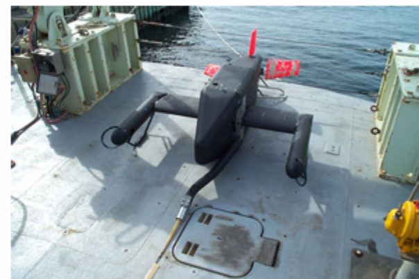
The Video Plankton Recorder attached to a winch cable on the deck of the R/V Atlantis at the WHOI dock. Credit: C. S. Davis @Woods Hole Oceanographic Institution.
