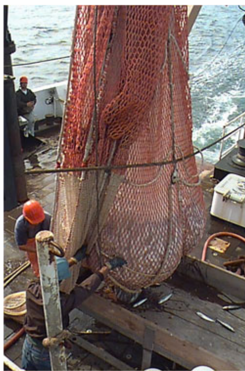
Figure 6. Emptying the cod-end of the High Speed Midwater Rope Trawl. Credit: NEFSC Photo Archives. Click to enlarge
