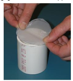
4. Press firmly around the edges until the silicone squeezes through the holes of the mesh. Smooth the silicone with your finger and then allow it to dry for about 30 minutes.
