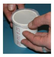
5. Insert the 4" PVC pipe into the PVC coupling making sure that the mesh covered end is orientated down. Force the 2 pieces together until the bottom of the 4" PVC pipe fits snugly against the inner lip of the coupling. To make sure that the PVC pipes are securely connected, place both hands on the upper pipe and lean down hard with your body. Or carefully bang the sieve on a hard surface a few times.
